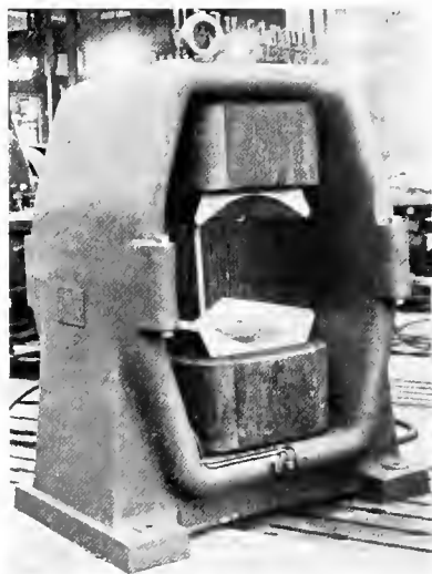
FIG. 20—FIELD OF EARLY ROTATING ARMATURE TURBO-GENERATOR
